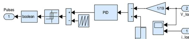
Figure 5. Feedback controller for the buck dc/dc converter
