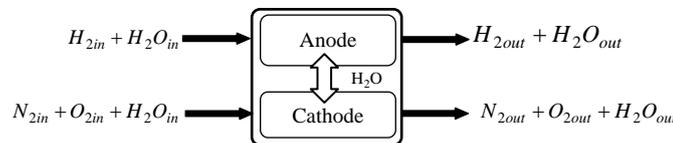
Figure 2. Illustration of gas flows of the PEMFC
