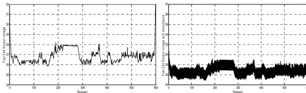
Figure 9. Fuel Cell Output voltages without disturbance and with disturbance
